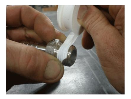
2. With the roll of thread tape in the position shown, hold the end of the tape flat against the thread with your left thumb while stretching the tape with the roll over the thread.
